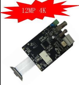
12MP 4K | SC5S226H19  | <b>12 megapixel 4K Ultra HD IP box camera module:</b> Sony starlight sensor IMX226 + Hisilicon Hi3619, illuminator: 0.001Lux@F1.2, color. 8 megapixel 4096*2160(4Kx2k) 25/30fps, alarm in/out, audio in/out, RS485, HDMI 1080P local output. SD card slot , auto-IRIS, support USB storage device H.265/H.264/MJPEG encoding. DC12V. PoE is optional. Support ONVIF and Hikvision protocol.                      |       |                  |
